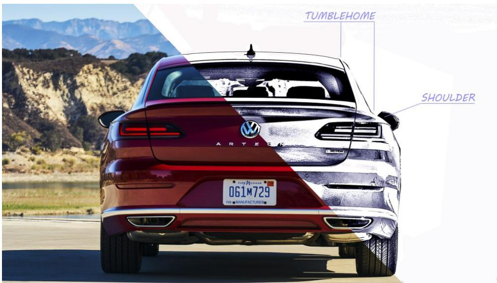
**Shoulder:** The side curve of a vehicle body, typically above the wheels. Many vehicles lack shoulders entirely, as the roof and sides meet in one
