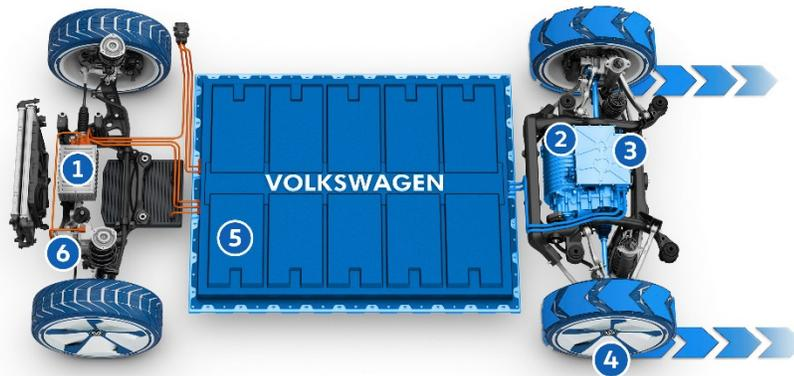
1. The low-voltage battery installed at the front will supply power to the vehicle electronic system and lights, among other things.
