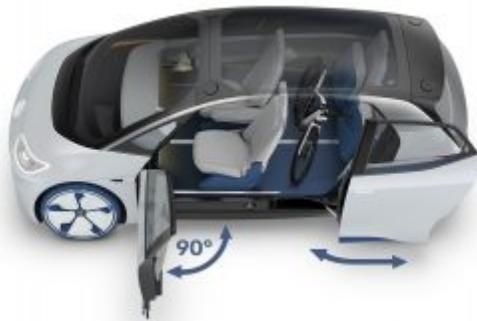
*The ID., one of the first cars based on the MEB, features classic doors at the front and sliding doors at the rear.*
